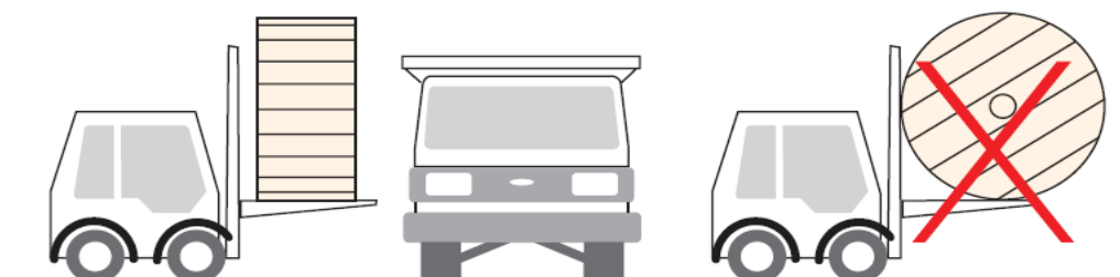
Lift drums on fork trucks correctly.
